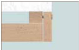
covering the hollow chamber with end plate
