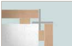
open corner with standard aluminium end plate
