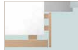
Different Resysta profiles can also be utilized for connections, e.g. window reveals with FP 200/5.
